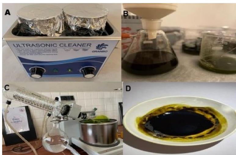
Fig 7. Schematic representation of the extraction and purification procedure for C. spinosa L.: (A) an ultrasonic process facilitates extraction; (B) solid-liquid separation is achieved via vacuum filtration; (C) the extract is concentrated using a rotary evaporator; (D) crude extract of C. spinosa L.
