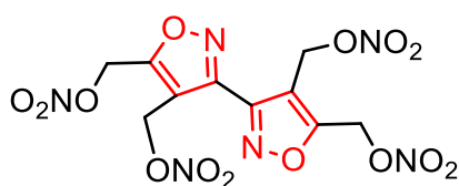
Fig. 12. Structure of 3,3'-biisoxazole-4,4',5,5'-tetrakis(methyl nitrate) TNBIO .
