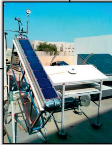
Fig. 12. Cooling system with convergent heat exchanger [5].
