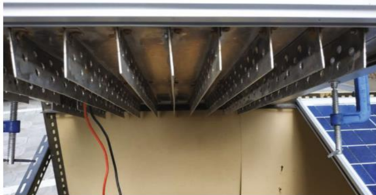
Fig. 4. Cooling system using heat sinks [11].
