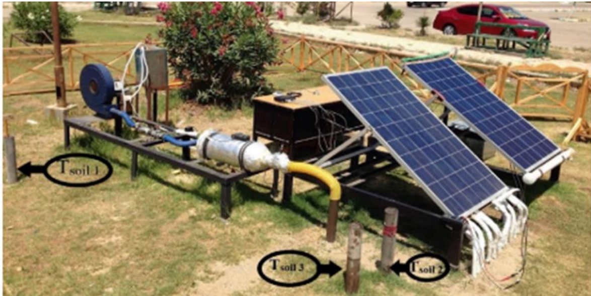
Fig. 9. Test stand of PV panel coupled with geothermal air cooling system [26].
